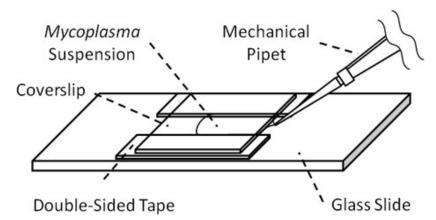
Figure 1. Tunnel chamber
