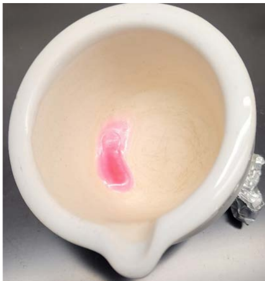
Figure 6. Appropriately poured TRIZol. TRIZol is confined to the sample. Crumbled aluminum foil is used to keep the mortar angled as TRIZol warms.
