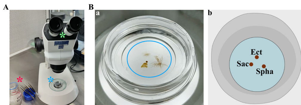
Figure 1. Brown algal tissue preparation for in vivo confocal microscopy. (A) Material used for mounting brown algal tissues. Stereoscopic microscope (green asterisk), sterilized forceps (red asterisk), glass-bottom cell culture dish, and coverslip (blue asterisk). (B) Brown algae mounted for in vivo confocal microscopy. a) Glass-bottom cell culture dish containing the labeled Ectocarpus sp., S. latissima , and S. rigidula placed in the middle and under the coverslip (outlined in blue) and filled with ASW. b) Schematic representation to localize the Ectocarpus sp. filaments (Ect), S. latissima embryo (Sac), and the S. rigidula filaments (Spha).
