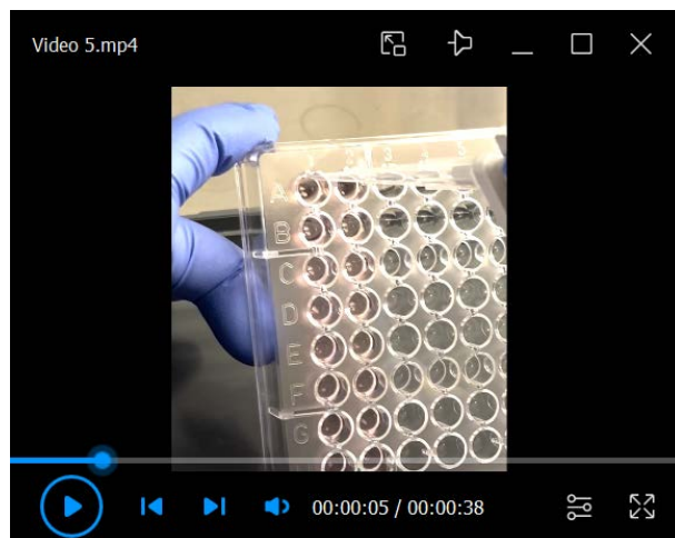
Video 5. Media change of murine blood vessel organoids (mBVOs) grown individually (every 48 h, from day 15 to day 30) (related to Figure 5). (A) Careful aspiration of the media from the top edge of the well, leaving minimal residual media. (B) Refreshing media (200 \mu L per well) using a multichannel micropipette and sterile reservoirs.
