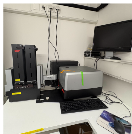
Figure 1. Stacker connected to a plate reader. The stacker connected to the plate reader handles up to 25 plates automatically. Plates are inserted into the input rack; then, a crawler moves the plate to the front, and the robotic arm removes the lid and places the plate onto the carrier. The carrier then inserts the plate into the plate reader, where the plate is shaken, and the optical density is measured. After the measurement, the plate is moved back, and the lid is added again and placed on the bottom of the output rack. When all plates are measured, they are automatically restacked to the input rack, and the process is repeated, allowing time series assays. The illustration (left) and photograph (right) show the stacker connected to the plate reader. A metal base plate fixes the distance between the two instruments.
