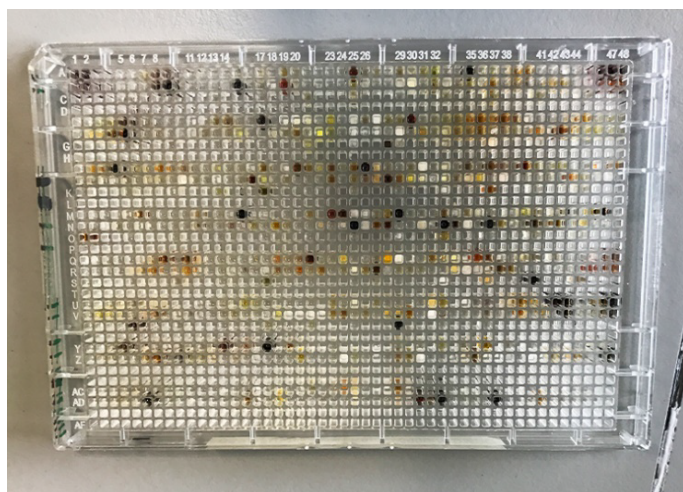
Figure 9. Plate with 768 compounds from the DSPL library. This set of compounds is used in fragment-based crystallographic screening for ligand identification.
