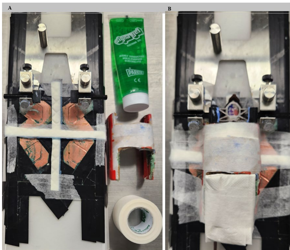
Figure 2. Final preparation of the physiological monitoring system before and after head-fixation of the mice for subsequent imaging, along with electrocardiogram (ECG) recordings. (A) Cutting and placing narrow strips of KRUUSE dental pads (0.5 cm wide) over each electrode area to absorb urine and excess gel, secured with 3M surgical tape. (B) Constructing and placing a custom half-tube cardboard tunnel (approx. 7.5 cm \times 2.5 cm) to provide restraint and comfort.
