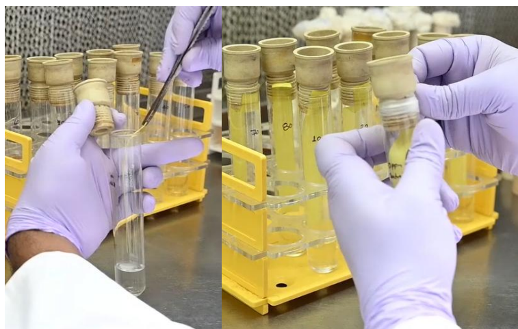
Figure 1. Insertion of the strip and sealing it with Suba seals and Parafilm
