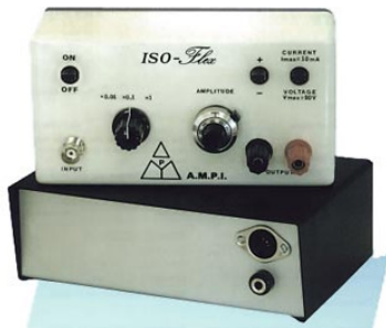
Figure 6. Isoflex stimulator. Stimulation can be given in positive or negative current or voltage. The stimulus max is 10 mA.
