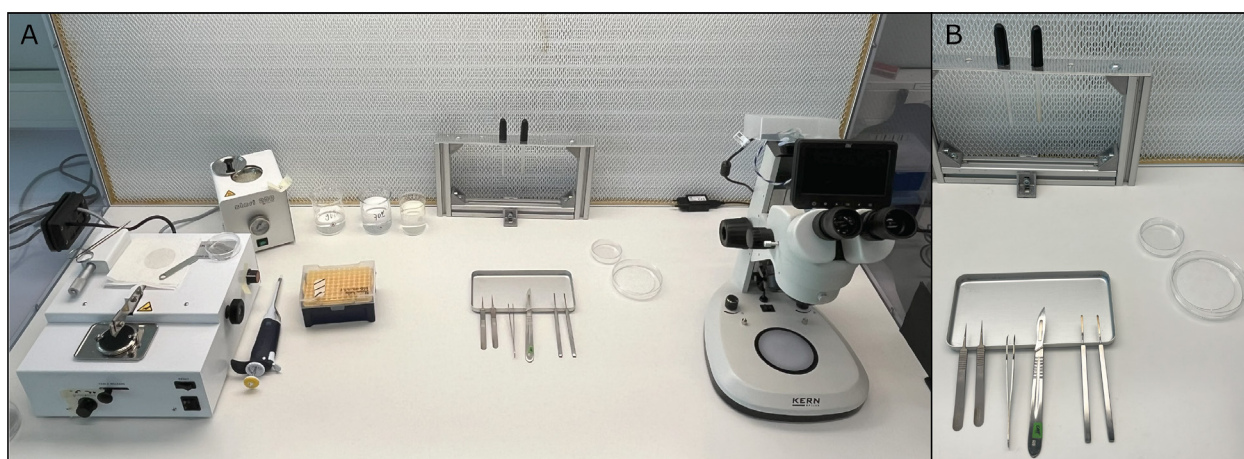
Figure 1. Dissection tools and working area. A. Overview of the working area and essential tools needed for dissection. From left to right: chopper, sterilizer, 200 µL pipette and tips, dissection tools, Petri dishes, and a microscope. B. Zoom-in view of essential dissection tools. From left to right: broken straight tweezers (two halves), bent tweezers, scalpel, two round spatula tools, and two glass pipettes in the rack smoothened using a Bunsen burner (one with a ~2 mm opening and one with a ~5 mm opening).
