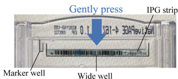
Figure 1. Preparation for native PAGE. Native PAGE gel with an IPG strip placed on top.
