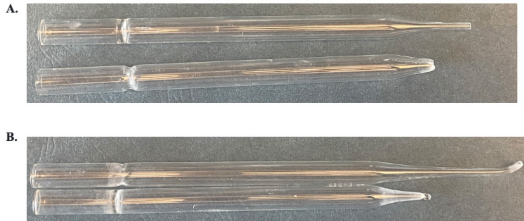
Figure 4. Glass Pasteur pipettes for X. laevis oocyte manipulation. A. Pasteur pipettes for moving oocytes. Top: some pipette taper remaining and a small opening; bottom: pipette taper removed and a larger opening. B. Pasteur pipettes for manual defolliculation. Top: more taper and longer length; bottom: less taper and shorter length.
