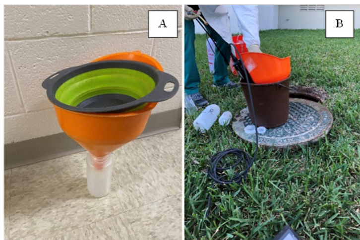
Figure 2. Configuration of sample collection in the field. A strainer and funnel are combined to facilitate the removal of large solids while guiding the wastewater into a bottle (A). In the field, the funnel, strainer, and bottle are placed within a bucket to capture spillage of wastewater, avoiding contamination of the surrounding ground (B). In the right panel, a water quality sonde (YSI Probe) is placed within a bottle inside the bucket, which facilitates the collection of physical-chemical water quality data in the field.
