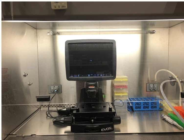
Figure 4. Image of microscope setup inside the biosafety cabinet for colony pickup
