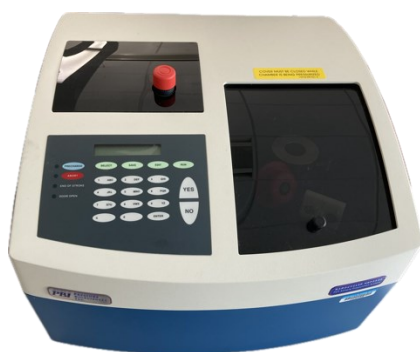
Figure 3. Pressure cycling technology (PCT) Barocycler instrumentation utilized for trypsin digestion of samples. The cycling methods can be programmed prior to use.
