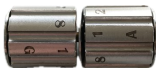
Figure 2. Microtube cartridges where up to 16 samples can be run on the pressure cycling technology (PCT) Barocycler for trypsin digestion.
