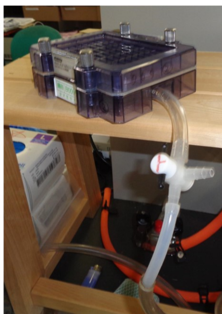
Figure 6. Slot blot apparatus on a stand; the large tube runs between the flow valve and water aspirator
