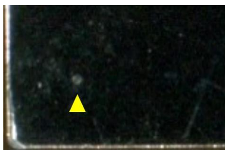
Figure 5. Example of a fiducial mark. The point highlighted by the yellow arrow is a laser etch mark that is created during building the custom MALDI target plate. This point should be visible both in the image and in the video feed of the MALDI-MS instrument. This etch mark is \sim 200 \mu\text{m} .
