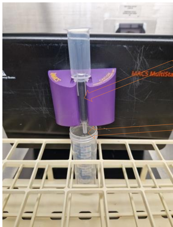
Figure 3. Setup of the LS column within the magnet; unlabeled cells go through, and labeled cells are retained by the magnetic field. Flush the LS column with 2 mL of washing buffer. Caution: This fraction contains the cDC2 population.
