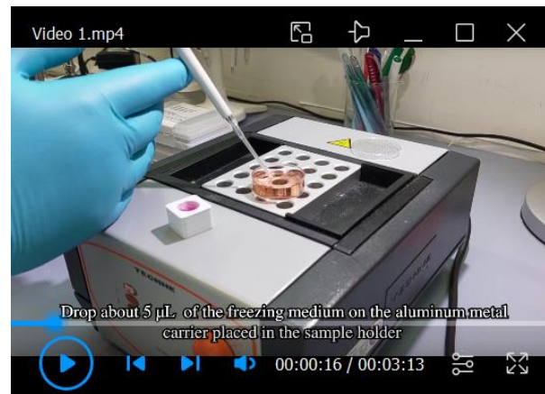
Video 1. Video tutorial showing the assembly of a sandwich for cryo-immobilization using the Wohlwend Compact 03 high-pressure freezer. This video corresponds to Figures 2 and 3.
