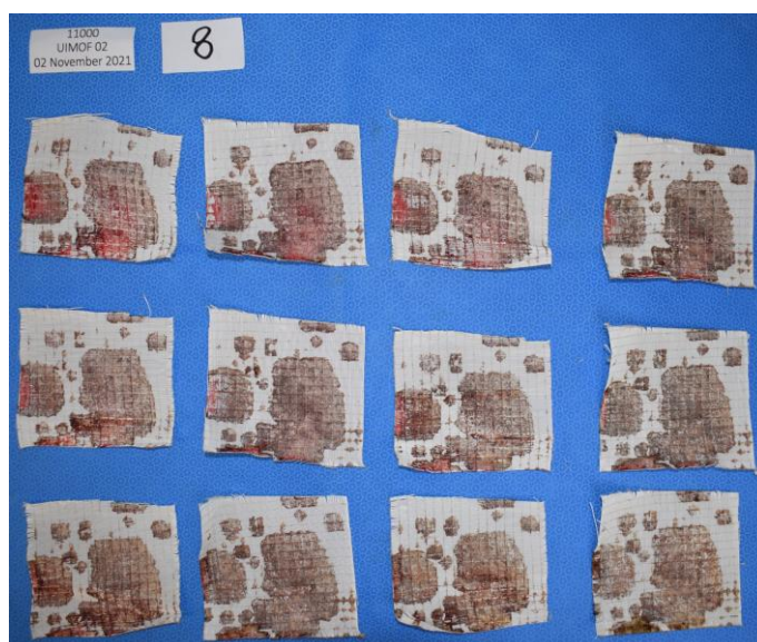
Figure 5. Layout example of membrane gas transfer fiber sheets for digital imaging
