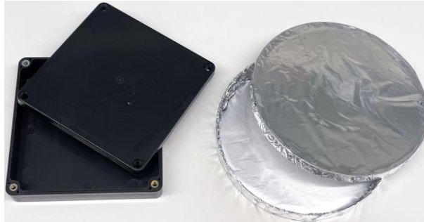
Figure 2. Examples of the chambers that can be used to protect optogenetically activated cell death effectors (optoCDE)-expressing cells from light
