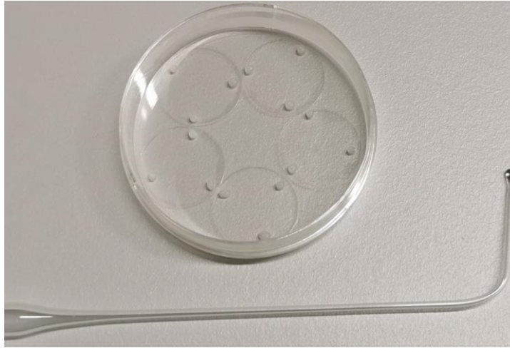
Figure 1. Fire-polished Pasteur pipette and 18 mm cover glasses with attached paraffin dots. Fire-polish the tip of the Pasteur pipette with a Bunsen burner. The tip should melt to form a glass bead with a diameter of approximately 2 mm (while heating the tip of the pipette, rotate it around the longitudinal axis to form a symmetrical bead), and the pipette should be bent by an angle of 50°–80° approximately 3 cm from the end of pipette.
