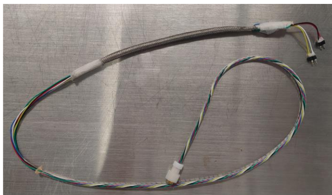
Figure 4. Electroencephalographic (EEG) patch cord. Patch cord with two connectors for EEG and electromyographic (EMG). The excess wires (here, blue and green) are taped against the metal braided sleeve.
