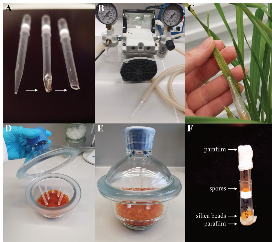
Figure 4. Spore harvesting procedure. A. Prepare the 1 mL filter tips. Carefully heat and flatten the tip. Cut the flattened part of the tip to generate a flattened opening. B. Attach a tube with an inner diameter of approximately 8 mm to the vacuum pump and insert the tip at the end of the tube. C. Start the vacuum (between 500 and 700 mbar is normally sufficient). Carefully move the spore hoover over the leaf surface to collect the spores in the filter tip. D. For drying, store the collected spores in the tips in an exsiccator filled with silica beads. E. Tightly close the lid of the exsiccator with parafilm during storage at 4 °C. F. 1 mL filter tip with harvested spores and silica beads, closed with parafilm.
