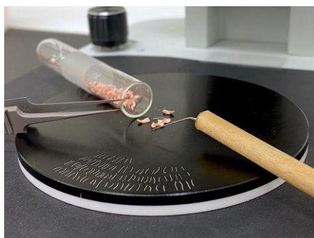
Figure 2. Manual isolation of individual freeze-dried muscle fibers. Isolation is performed under a stereomicroscope using Dumont forceps and custom needles created from sharpened sewing needles
