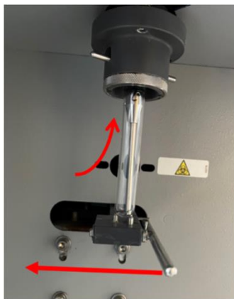
Figure 4. Flow cytometry sample insertion
