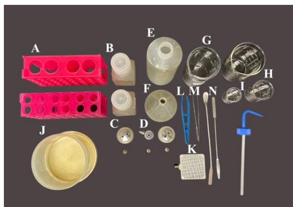
Figure 2. Materials to be autoclaved for 3D bioprinting with the aspect. A) Conical holders (2×); B) 125 mL Nalgene bottles (2×); C) 125 mL Nalgene bottle printing lid and tubing fastener (2×); D) 15 mL bioink conical printing lid and tubing fastener; E) 500 mL squirt bottle; F) Funnel; G) 200 mL beaker (2×);
