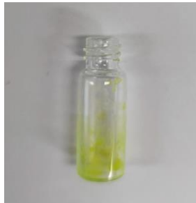
Figure 1. Image showing dried lipid layers adhered to the wall of a glass vial. 1% DiO dye is included to label the lipids for better demonstration.
