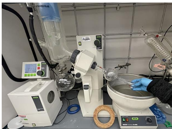
Figure 1. Solvent evaporation by rotary evaporator
