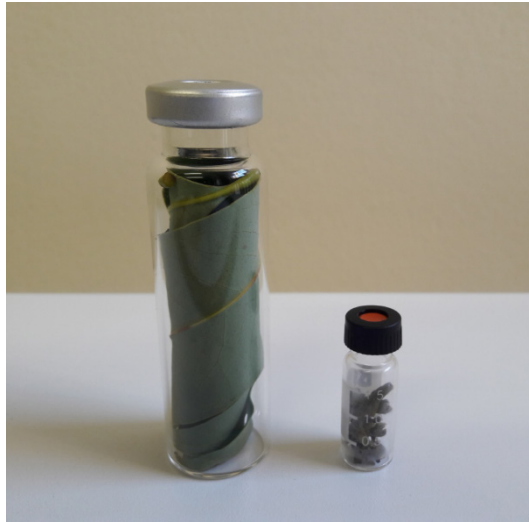
Figure 5. Leaves and buds sealed in 20 mL (left) and 2 mL (right) vials, respectively
