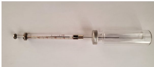
Figure 8. Use of a 100 \mu\text{L} syringe to dilute \text{C}_2\text{H}_4 gas in a headspace vial
