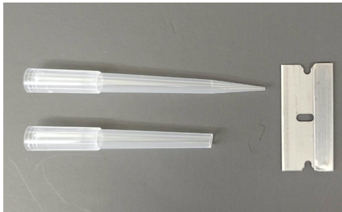
Figure 4. Preparing pipette tips for viscous solutions. Comparison of an uncut 1,000 \mu L pipette tip (top) and a tip with approximately 2 cm cut off with a razorblade (bottom).
