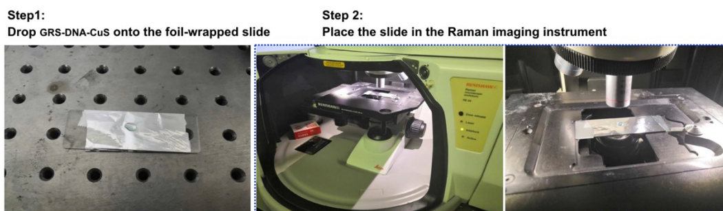
Figure 3. Process for measuring Raman signal intensity of GRS-DNA-CuS nanodandelions
