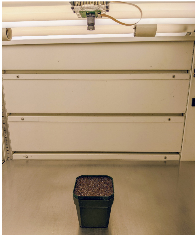
Figure 2. Setting up camera location within the growth cabinet and placing a representative pot below for image optimization
