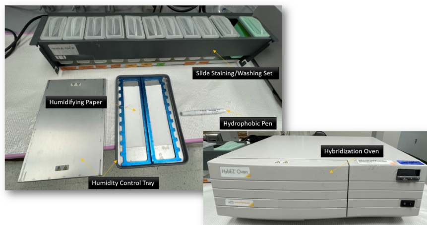
Figure 2. HybEZ II system. Hybridization oven, humidity control tray, humidifying paper, slide staining/washing set (EZ-Batch wash tray and EZ-Batch slide holder), and hydrophobic pen indicated.
