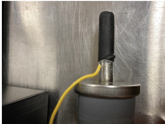
Figure 9. Wire soldered to the water-filling tube. Picture showing the wire [connecting the capacitive touch sensor (MPR121) to the water-filling tube] soldered directly to the water-filling tube.
