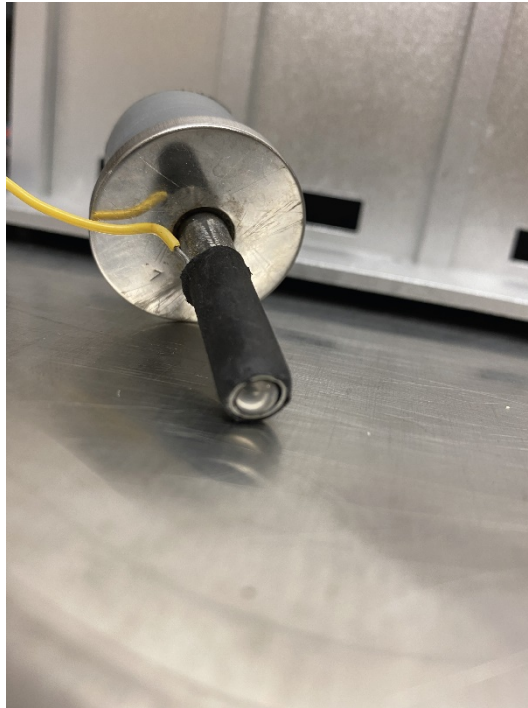
Figure 10. Heat shrinking tube. Picture showing the heat shrinking tube covering the water-filling tube and the wire connecting the capacitive touch sensor with the tube.
