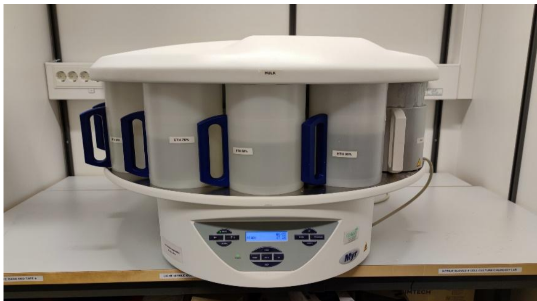
Figure 1. Spin Tissue Processor (STP 120) showing individual containers numbered 1-12 and the programmable interface.
