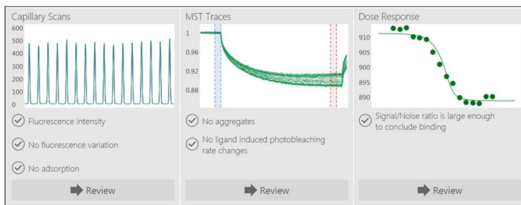
Figure 2. Capillary scan, microscale thermophoresis (MST) traces, and dose response of a representative experiment.
