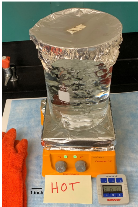
Figure 2. Syrup at rolling boil and treated with citric acid.
