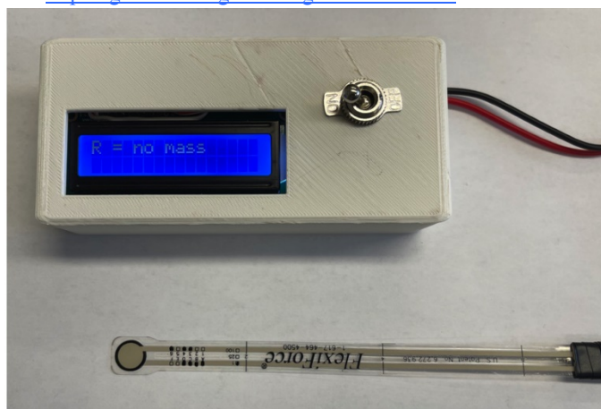
Figure 16. Completed pressure sensor device with portable housing unit.
