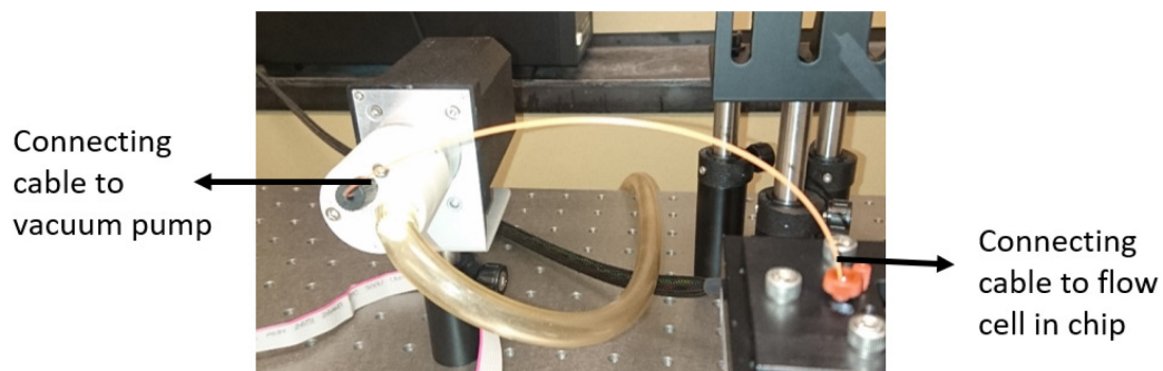
Figure 7. Vacuum pump connection to the microfluidic chip device.
