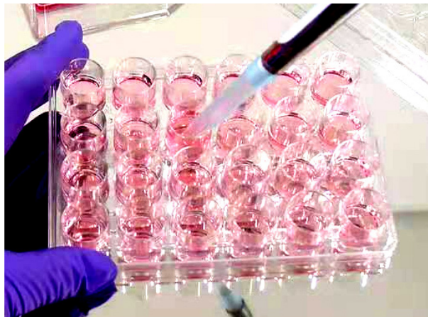
Figure 3. Aspiration and release of the medium should be performed at the side of the wells.
