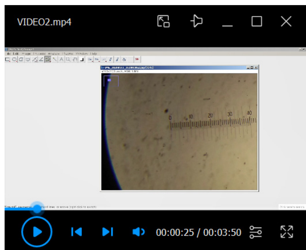
Video 2. Determination of average Feret's pore diameter using ImageJ tool
