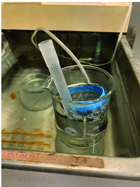
Figure 3. Beaker filled with ACSF solution and a floating net for incubation of brain slices at 33°C
