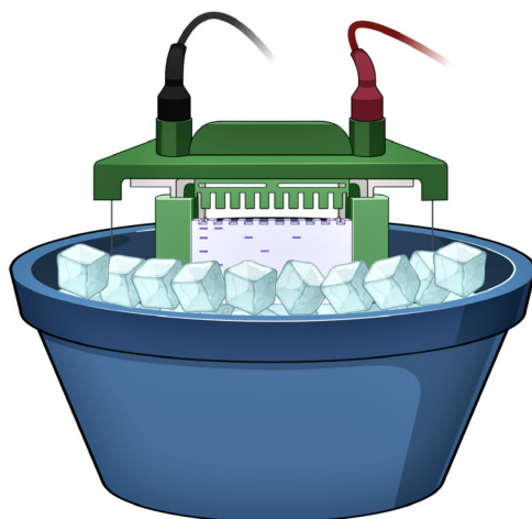
Figure 2. Schematic diagram of native-PAGE set up
