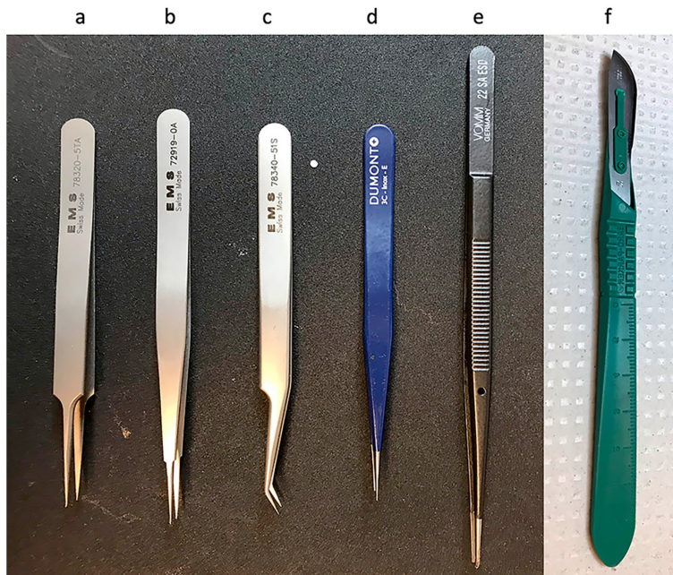
Figure 1. Tools for sample handling. a-c. Sharp-point tweezers for sample handling (Section A Steps 4-5). d-e. Insulated tweezers for frozen sample recovery and transfer (Section B Steps 4-9, and Section C Steps 6-7). f. Crimping tool: #20 scalpel manually blunted by rubbing the blade gently on a metal surface (McDonald et al. , 2010).
