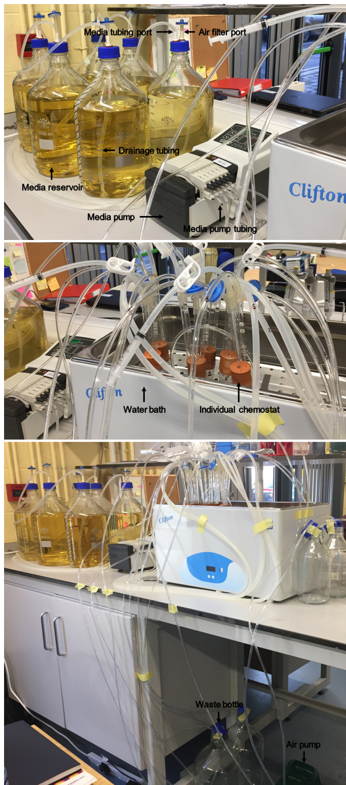
Figure 3. Illustration of the multiplex continuous culturing system. The constituents of the system and their connections are depicted.
