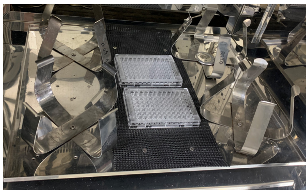
Figure 4. Incubating the E. coli -containing U-bottom 96-well microplate in an incubator. Remove some of the flask holders and replace the space with an anti-slip pad. Fix the anti-slip pad with screws. The anti-slip-containing area is ready for incubating the 96-well microplate.
