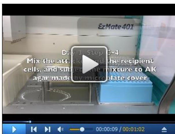
Video 1. Mix the attacker and recipient cells and subject the mixture to AK agar. Use the automated pipetting system to add 10 \mu l overnight-cultured E. coli (upper right Block C) into the A. tumefaciens -containing 2.2-ml 96 deep-well microplate (upper left Block A). Mix the bacterial suspension 10 times and drop 10 \mu l mixture onto the AK plate (lower left Block B).
