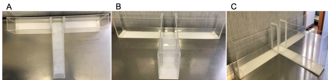
Figure 1. T-maze apparatus. Photographs show the top view (A), front view (B) and side view (C) of the T-maze for mice used in Leggio et al. (2019).
