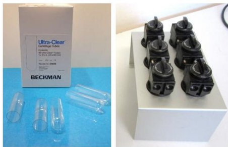
Figure 2. Ultraclear thick ultracentrifugation tubes should be loaded into the tube holder before mass equilibration for ultracentrifugation
