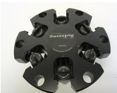
Figure 3. Ensure loading SureSpin tubes in the right socket to avoid equilibrium troubles
