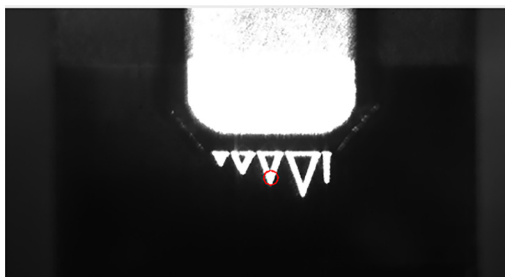
Figure 3. CCD picture of the cantilever tip in the AFM experiment. The triangle which the red ring located is D tip. The red ring points out the laser radiation position on D tip.
